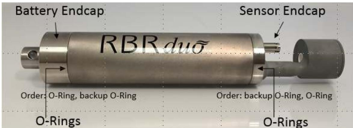
2. **O-rings should be seated in a clean and un-scored groove.** Carefully inspect the O-ring grooves and the logger body for nicks and scratches. If any are found, contact RBR for advice. Gently clean all grease and dirt from the O-ring grooves, end cap surfaces, and logger body end bores.
