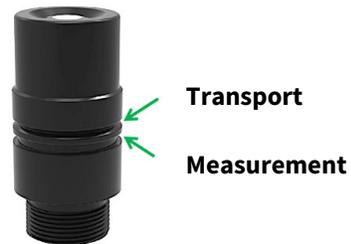
During transportation or storage, move the red O-ring of the Oxyguard sensor to the "Transport" position, closing off the port on the side of the cell.
