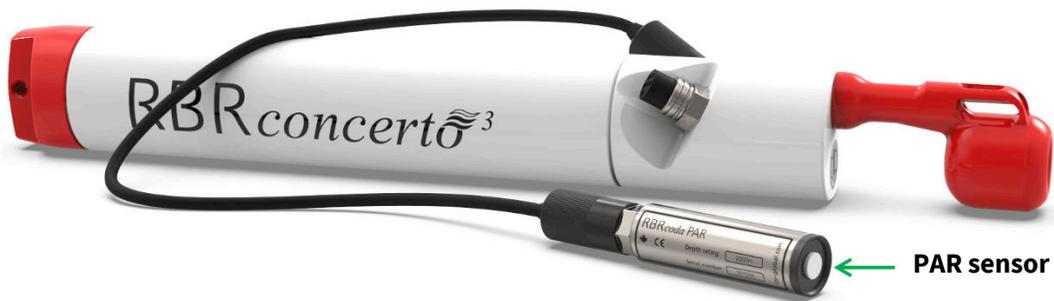
**RBRconcerto<sup>3</sup> C.T.D.PAR with a cosine PAR sensor (RBRcoda<sup>3</sup> PAR)**
