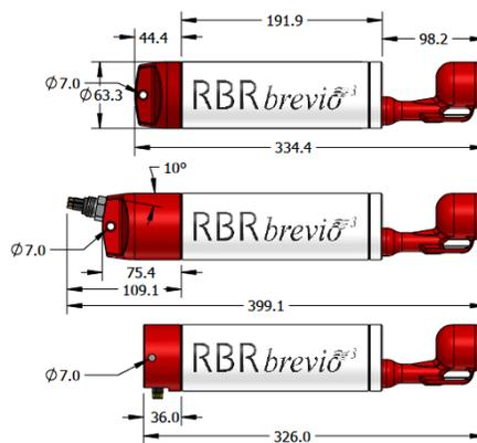
**RBR*brevio*<sup>3</sup> dimensions with three different battery end-caps**
