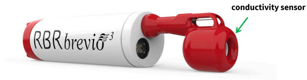
**RBR*brevio*<sup>3</sup> C.T.D with a conductivity sensor**
