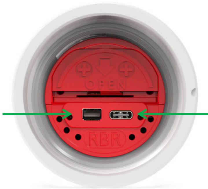
Left: mini-display port, right: USB-C port
