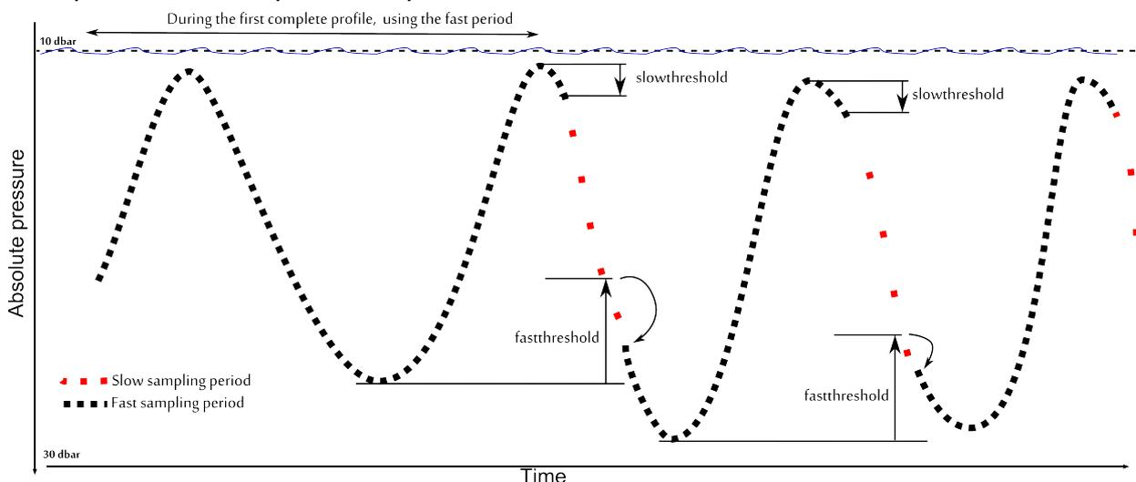
The next picture shows how the directional dependent sampling would behave in the case of a profile much shorter than the previous one. In such a case the logger would detect an upcast while slow sampling and would then go back to the fast sampling mode.
