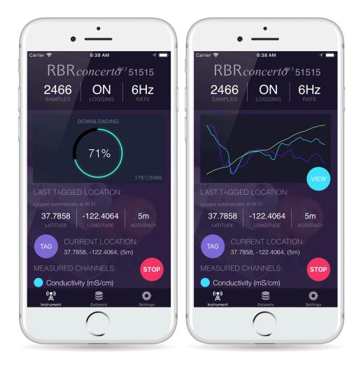
After connecting to the logger, you are automatically in the **Instrument** view of the app. The different views you can go to are **Instrument**, **Datasets** and **Settings**, located at the bottom of the screen. Tap **Datasets** to view a list of local datasets, and (optionally) remote datasets you have stored in your Dropbox account. This is also how you can share/ upload and view your data, explained more later.
