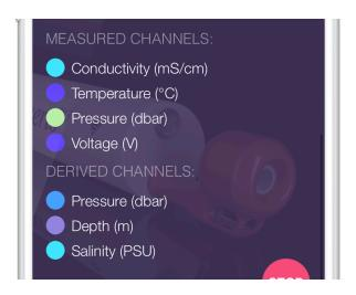
Scrolling to the bottom of the Instrument tab reveals the instrument's Measured and Derived Channel lists along with their units of measurement. The colored circle to the left of each channel indicates the sparkline color used to represent the latest readings from that channel.
