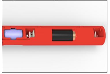
To insert the battery, press the battery into the battery holder, ensuring it is correctly oriented with the negative terminal placed towards the electronics. The label in the logger indicates proper battery placement.
