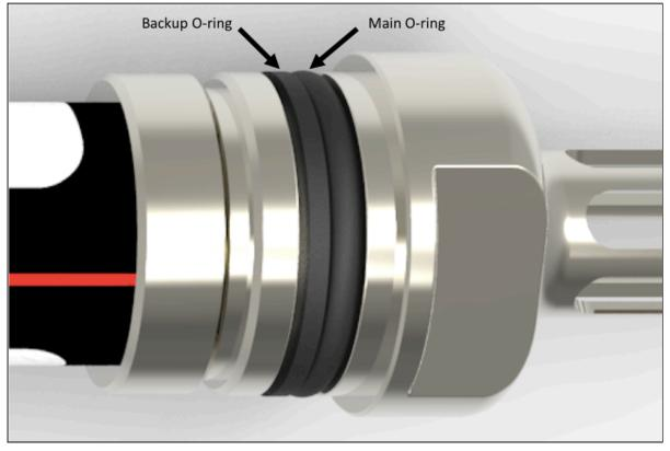
Before you remove the O-rings from the RBRsolo or RBR*duet*, make yourself familiar with their orientation and location. Inspect the new O-rings provided in the loggers support kit – there are two types. The back-up O-ring is a flat O-ring with a concave channel on one side. The main O-ring is round.
