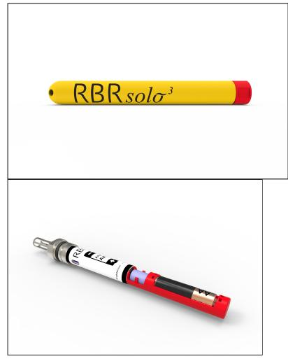
Closing the logger is exactly the reverse of opening it. Remember to keep the O-rings clean and avoid scratching the O-ring mating surfaces. Carefully inspect the O-rings before deploying the logger. Do not use excessive force when tightening the end sensor end; hand-tight is quite sufficient, as the seal depends upon the O-rings, not the end cap tightness.
