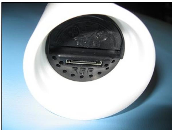
Closing the logger is exactly the reverse of opening it. Remember to keep the O-rings clean and avoid scratching the O-ring mating surfaces. Carefully inspect the O-rings, as described in the Inspecting the O-rings section (p.10), before deploying the logger. Do not use excessive force when tightening the end cap; hand-tight is quite sufficient, as the seal depends upon the O-rings, not the end cap tightness.
