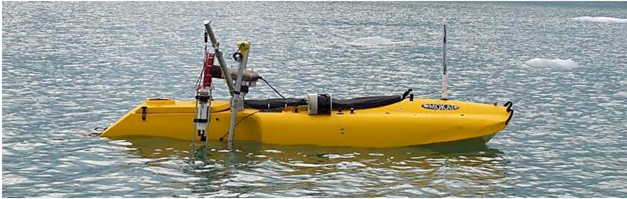
The WHOI Jetyak with mounted instrumentation including an RBRconcerto CTD (white). Credit: C. Richards.*
