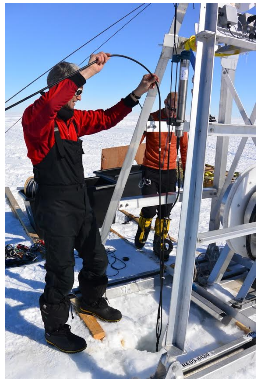
Keith Nicholls attaching the thermistor cable to the main mooring cables.
