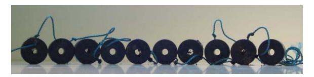
Figure 4. The samples with the central holes view after receiving them back in RBR. From left to right: #1 – non-coated, #2 – coated, #3-non-coated, #4 –coated, #5-non-coated, #6-coated, #7-non-coated, #8-coated, #9-non-coated, #10 -coated
