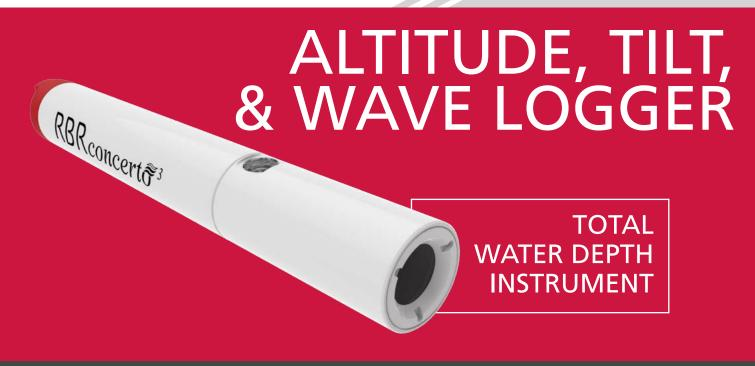
The RBRconcerto<sup>3</sup> D.alti.tilt is a unique data logger dedicated to total water depth. Equipped with a 3-axis tilt sensor and a 200kHz altimeter, the logger provides complete distance-to-surface and distance-to-bottom data. The instrument also includes a depth channel capable of both continuous and intermittent bursts. The RBRconcerto<sup>3</sup> D.alti.tilt is available in a configuration that supports wave measurements up to 16Hz.
