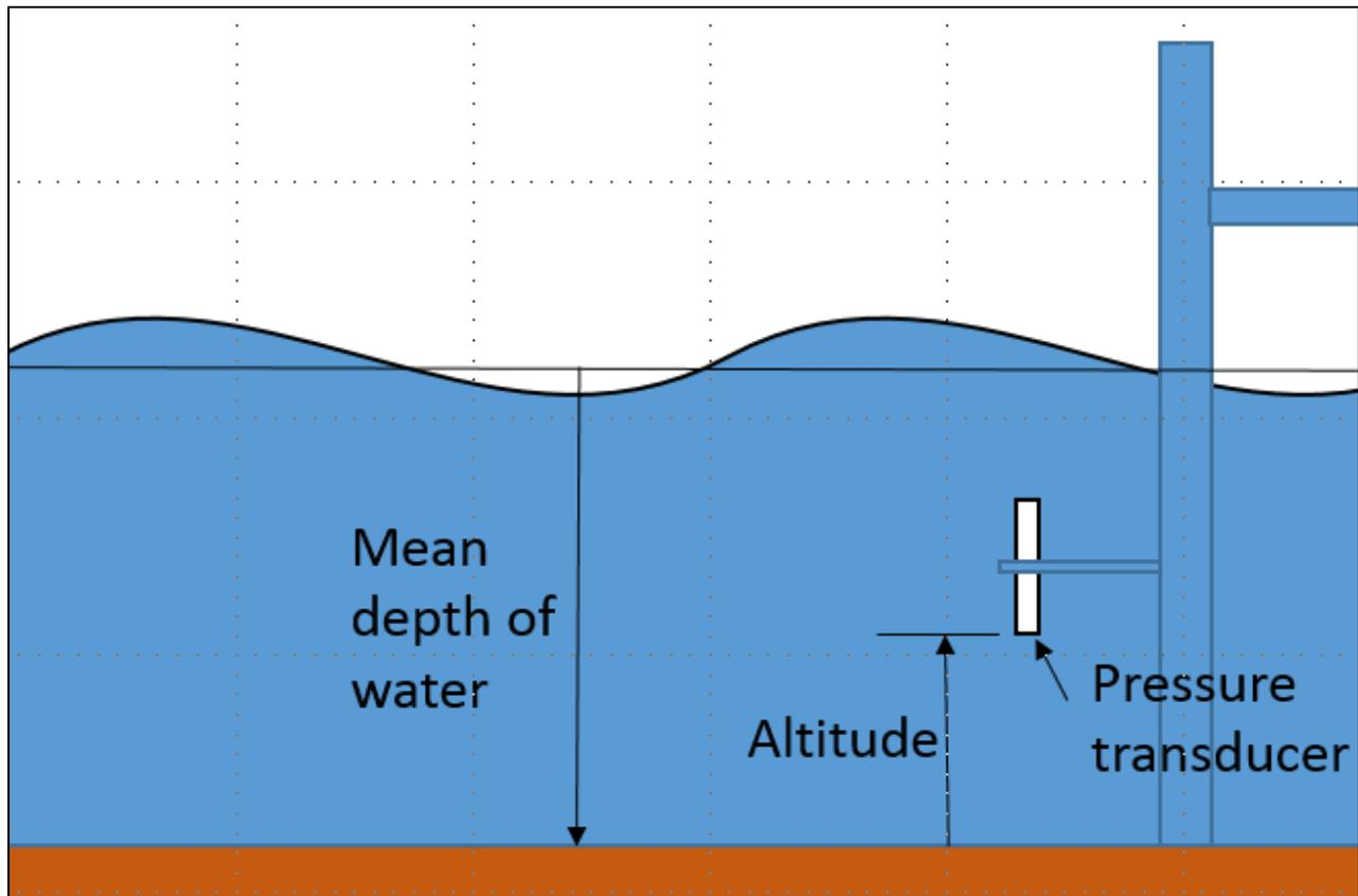
Figure 1. Logger positioning
